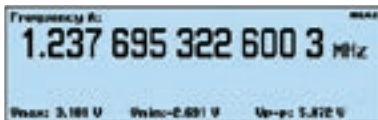
Figure 1: Measurement speed as high as 12 digits/s and a 14-digit display resolution is standard.
